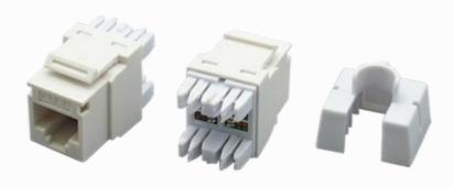
Category 6A unshielded keystone jack supports the 10/100/1G BASE-T Ethernet, as well as advanced 10G BASE-T Ethernet, meets and exceeds ANSI/TIA-568.2-D and ISO/IEC 11801 2nd edition standards. By special designed housing and installation the jacks on a staggered 24-port 1U patch panel, it minimizes additional AXT from neighboring connectors, and provide transmission performance beyond 500MHz and Alien crosstalk requirements
