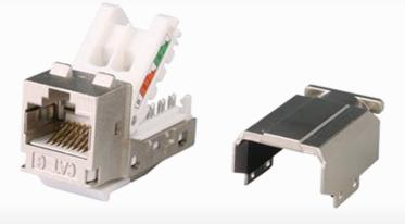
Category 6 shielded keystone jack is designed for superior performance and easy assembly, meets and exceeds ANSI/TIA-568.2-D and ISO/IEC 11801 2nd edition Category 6 standards, supporting Gigabit Ethernet application and beyond. Narrow width design fits 24 ports in one unit panel for most efficient use of 1U panel.
